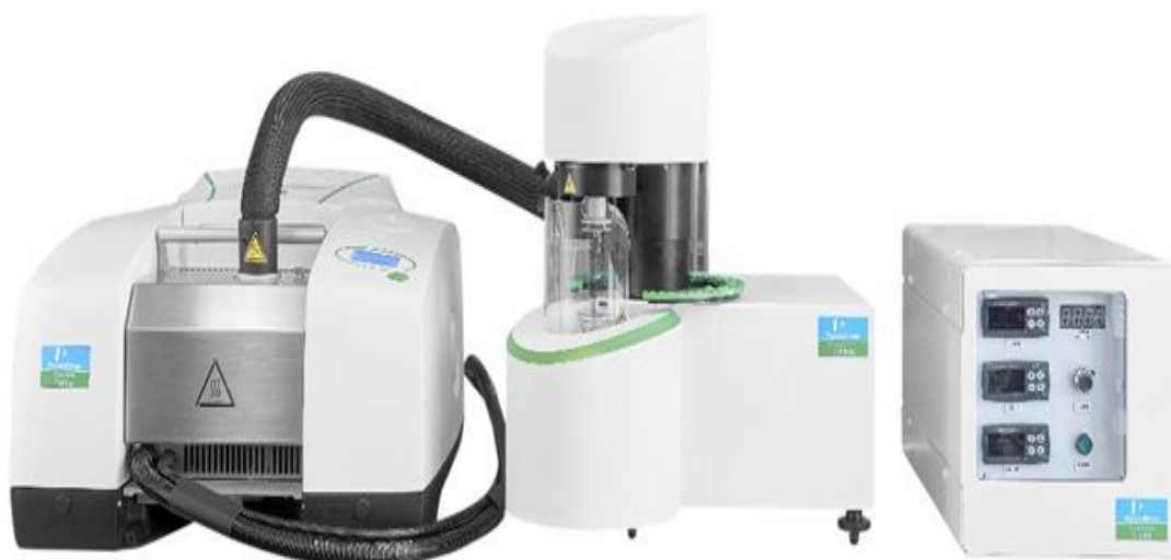
Fig. 1: Schematic diagram of TG-FTIR.
